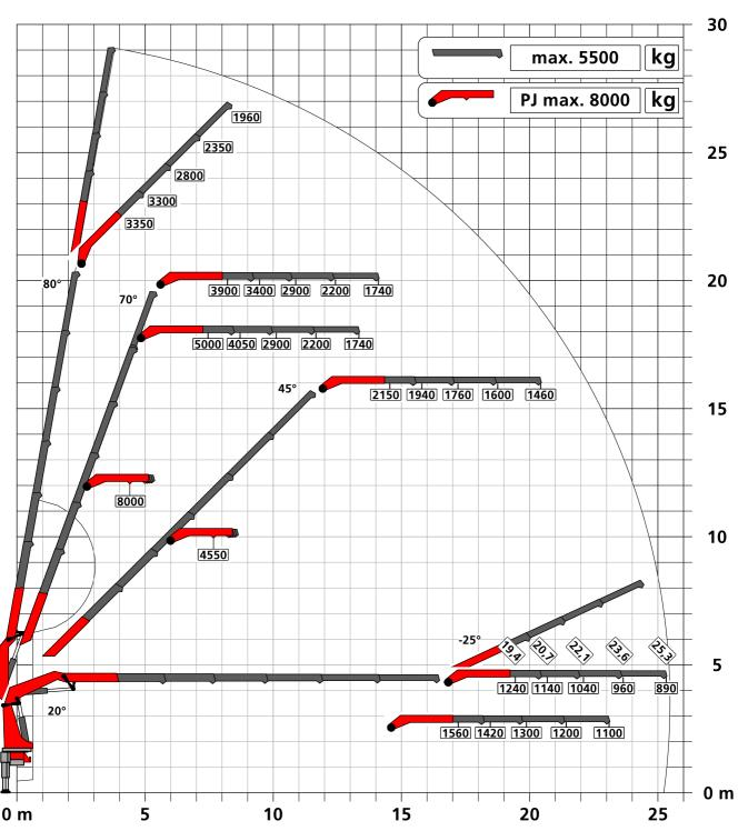
The load capacities as per chart are not reached when using hose equipment on the Fly-Jib.
